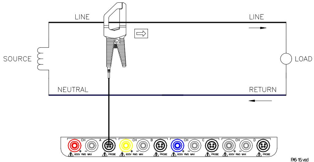
**NOTE:** The connection shown above is not recommended without a voltage connection to ensure frequency synchronization. If this configuration is used, then an internal frequency reference must be entered. Refer to pages 5-14 to 5-16.
