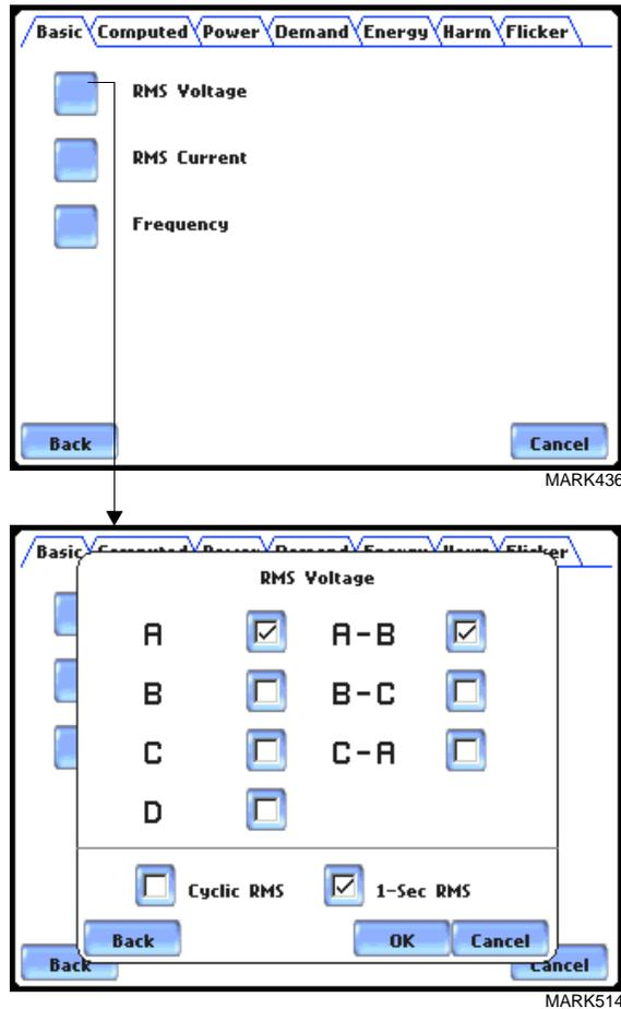
**Cyclic RMS:** RMS values are computed over 1 power frequency cycle (16.67 msec @ 60 Hz) in 1/2 cycle steps (every 8.33 msec). The min/max/avg of these cyclic values are continually updated and saved every user-programmed journal interval (see Chapter 6 Advanced Setup Options - Journal Interval for Timed Readings on page 6-21).
