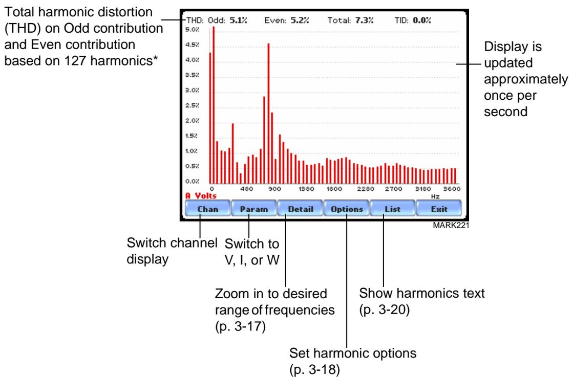
*\*The odd contribution is the square root of the sum of the squares of the relative amplitudes of harmonics 3, 5, and 7 through N-1, where N is a function of sampling frequency. The even contribution is similar for harmonics 2, 4, and 6 through N. Total value is the square root of the sum of the squares of the odd and even distortions.*
