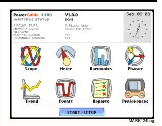
NOTE 1: The message MONITORING STATUS: DONE appears to indicate that monitoring is completed and active recording is disabled.
