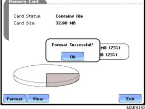
STEP 3: The 4400 lists data file names stored in card, along with file size, time and date when data was recorded. The text color indicates the type of file: black is for data file (.ddb), green is for setup file (.set), and red is for an unknown file.
