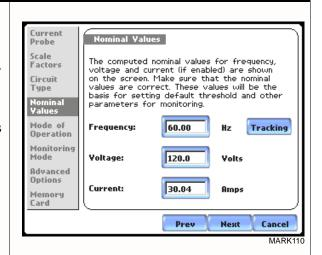
NOTE: Make sure that the nominal values computed by the 4400 are correct. Nominal values are used as basis for setting default thresholds and other parameters for circuit monitoring.
