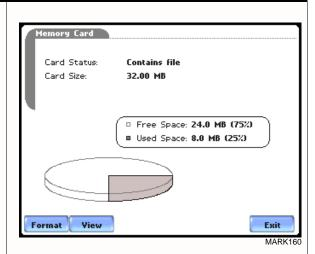
NOTE 1: The 4400 does not support file fragmentation. When creating a file, it will take the largest continuous block and use that size block for data storage. Deleting files from data card is not recommended. Whenever possible, transfer the files to a computer and then reformat the card using the 4400 when there is no more space available to begin new data storage.
