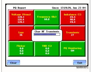
NOTE: An activity indicator periodically appears in the middle of the screen signifying that data monitoring is on and the unit is actively characterizing events.
