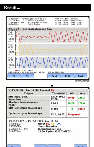
NOTE: The event textual summary is color coded. Red indicates the threshold value(s) and parameter(s) that are out of limits. Green indicates the measurement parameters that are within limits.
