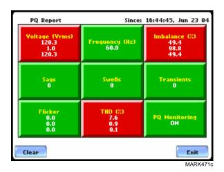
NOTE: The three values reported within a red or green square in the PQ Report screen refer to measurements on channels A, B, and C respectively. The measurement values for each channel are updated approximately once per second while monitoring is on.
