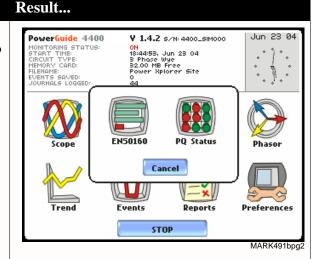
STEP 2: The panel is color coded. Green indicates the parameter is within limits and/or no events have occurred since the panel was last cleared. Red indicates the parameter is out of limits and/or events have occurred since the panel was last cleared.
