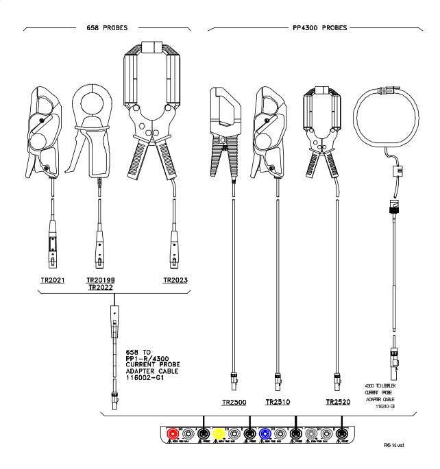
NOTE Current probes TR2500 can be used interchangeably with TR2500A, TR2510 with TR2510A, and TR2520 with TR2520A
