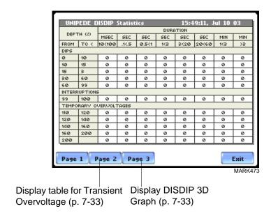
RMS Event Count: The table shows rms variations of specified range of magnitude and duration, also called bins. For example, an rms variation with a magnitude of 80-90% of nominal and 1-5 cycles in duration is one bin, whereas 80-90% and 10-30 cycles is another, 70-80% and 10-30 cycles is another, and so on. Each time that the characteristics of an rms variation match the criteria of the bin, the counter is incremented. RMS phenomena are typically found in bin groupings such as:
