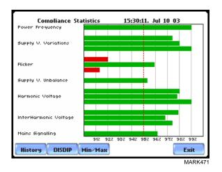
The bar chart indicates the percentage of the intervals passing the specified compliance criteria. The color of the bar indicates the compliance status. A green bar indicates that the parameter is within compliance. A red bar indicates that the parameter does not comply with EN50160 Standard. See below for the description of each measurement parameter. For the QOS compliance limit values of EN50160 parameters, refer to the table of Compliance Limits on page 7-24.
