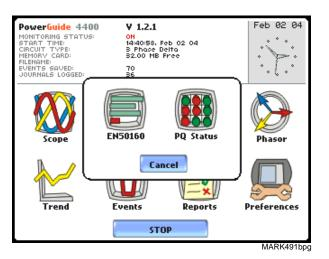
EN50160 displays statistical reports on QOS compliance. Statistical data is calculated on the required parameters specified in EN50160 over a one week interval to produce a PASS/FAIL decision of compliance. The standard monitoring period is one complete week, beginning Sunday 00:00 (midnight). Monitoring periods of less than one week will render an evaluation status that is Incomplete and compliance marked as Undetermined. Press EN50160 to access the EN50160 statistical reports. See page 7-22.
