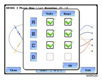
Press to enable/disable the parameter/channel for display in the animated phasor rotation. Any of the following will turn channels on/off:
