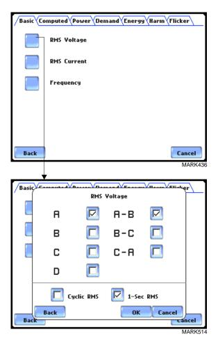
**Cyclic RMS:** RMS values are computed over 1 power frequency cycle (16.67 msec @ 60 Hz) in 1/2 cycle steps (every 8.33 msec). The min/max/avg of these cyclic values are continually updated and saved every user-programmed journal interval (see Chapter 6 Advanced Setup Options - Journal Interval for Timed Readings on page 6-21).
